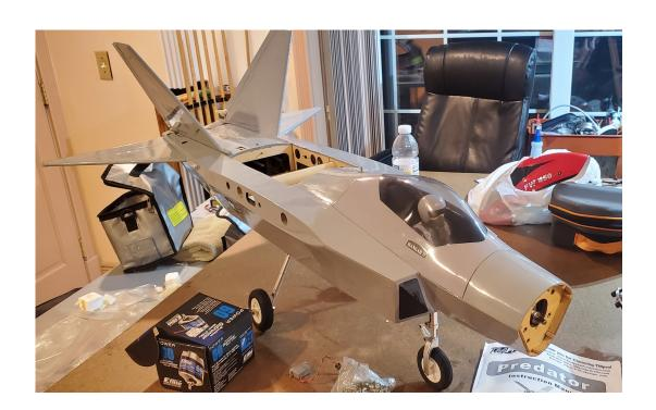
Just a photo of a brand new Hanger 9 F-22 Raptor, being converted from glow 35 to a Rimfire 60 with a 80A esc, also retrofitted with custom made electric retracts and full 90 degree deflection on most surfaces. A custom paint/Camo pattern coming next.
