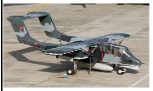
The **North American Rockwell OV-10 Bronco** is an American twinturboprop light attack and observation aircraft. It was developed in the 1960s as a special aircraft for counter-insurgency (COIN) combat, and one of its primary missions was as a forward air control (FAC) aircraft. It can carry up to 3,200 lb (1,450 kg) of external munitions, internal loads such as paratroopers or stretchers, and loiter for three or more hours.
