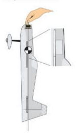
Check the vertical balance of your smaller 3D models by supporting them from the propelier shaft. When possible, move things toward the top of the fuselage to achieve a better vertical balance and a more stable, less-demanding hover.
