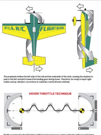
Briefly pumping the throttle higher while hovering improves control authority without maintaining the higher throttle positions long enough to cause the plane to climb.
