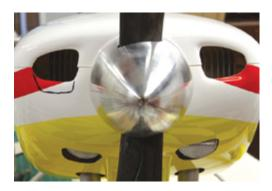
2 My first step is to increase the airflow coming into the cowl by enlarging this front opening. By increasing the opening size in a downward direction, I also center my cowl entry hole to the engine's cylinder head.
