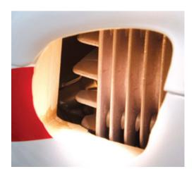
10 As you can see from this view, I now have a larger opening for air to flow in and help cool the motor. All air that now flows in through the cowl opening has to go over the engine cylinder head on its path through the engine compartment. That makes efficient use of all cooling air, resulting in a much lower overall engine temperature. This is a simple addition to any engine compartment that will always improve your engine's performance and efficiency. Try it and enjoy!
