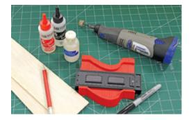
1 The materials I used include (left to right) 3/32 balsa wood for the ducting or baffles, hobby blade, 5-minute epoxy (or 30-minute epoxy), microballoons, pattern transfer gauge, felt-tipped pen and a Dremel tool with drum sander bit.
