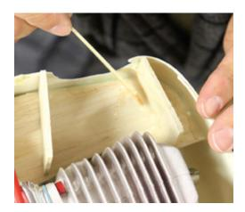
9 All that is left to do is to mix up some epoxy and microballoons and apply it to all of the corners of my ducting/baffles. I added some triangle balsa to the bottom of the ducting where it attached to the cowl for added support. Make sure you work with fresh epoxy; if it starts to cure, mix a new batch. Fresh epoxy will flow into the wood fibers and make for a stronger bond. I only mixed up enough epoxy for each corner; I ended up mixing about 12 small portions of epoxy for this side alone.
