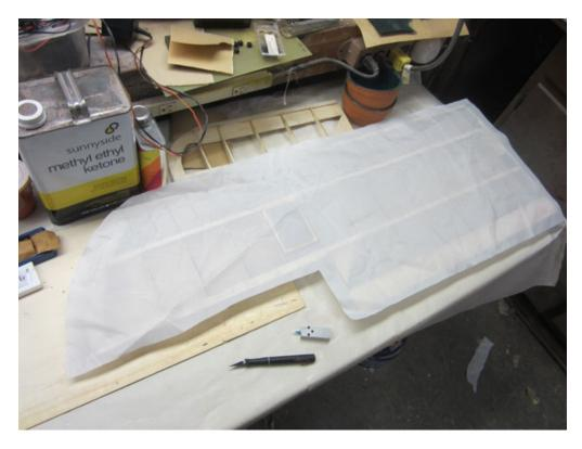
Start by applying a coat of Poly Tak adhesive all around the outer edges of the wing panel and let dry. Now cut the fabric to the rough size for the part. I make it about an inch oversize all the way around. Be sure to have a clean work surface. I use drafting vellum as I have a large supply of it.
