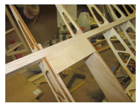
Sand all the wing ribs, spars, attachment plates, wing tips etc., smooth and then clean up any dust.
