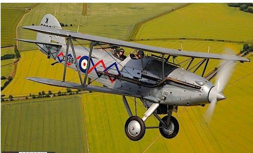
(March): **Hawker Demon**(Left): A fighter version of the highly successful 1928 Hawker Hart day bomber, the Demon two-seat escort fighter went into service in 1933. The Osprey was a navalised reconnaissance version for service with the fleet. (specifications) *Span:* 37ft 3in, *Length:* 29 feet 1 inch, *Engine:* Rolls-Royce Kestrel II , 851hp, *Max Speed:* 181 mph at 15,000ft, *Ceiling:* 24,500ft, *Armament:* 2x Vickers MG, 1x Lewis MG
