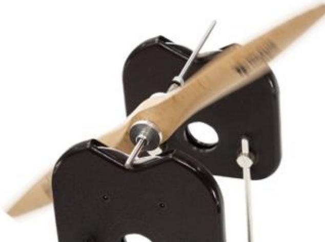
The second step is to place the prop on the balancer in the horizontal position to find out which side has the heavy blade.
