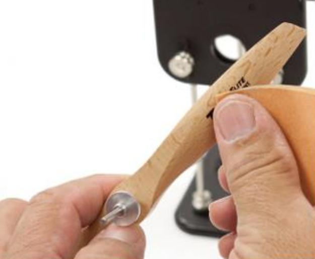
**3: REMOVING MATERI** Two methods are commonly used to balance the propeller. The first involves lightening the heavy blade until the propeller balances close to the horizontal position. Use a razor blade or sand paper to remove small
